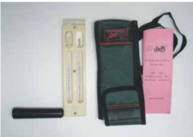
Whirling hygrometer or Psychrometer to monitor the temperature and RH
