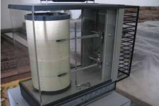
Thermo-hygrograph placed in a gallery to continuously record temperature and relative humidity
