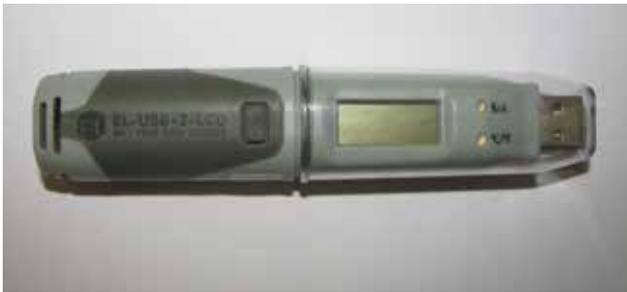
Digital USB Data-logger to record the temperature and relative humidity
